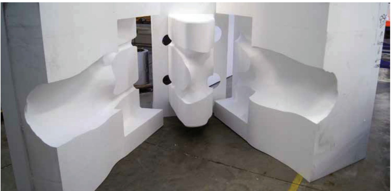
Figuur 8 Twinplast-EPS Mal
